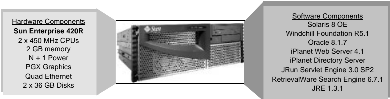
Figure 5 1-200 concurrent user Pilot or Development/Test configuration using a Sun Enterprise 420R server, scalable to 500 concurrent users
