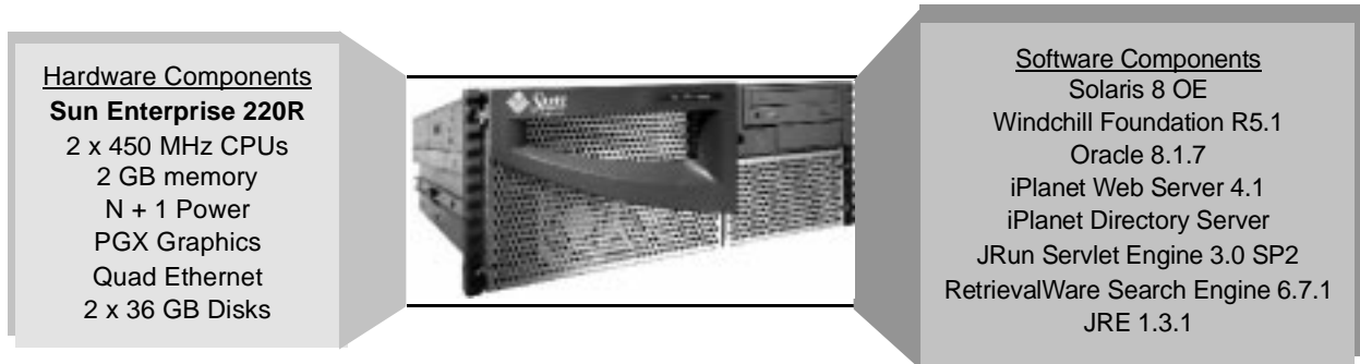
Figure 4 1-200 concurrent user Pilot or Development/Test configuration using a Sun Enterprise 220R server
