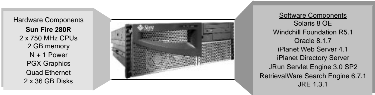
Figure 7 1-300 concurrent user Pilot or Development/Test configuration using a Sun Fire 280R server
